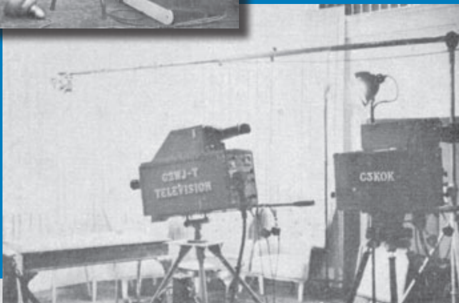
The Studio, showing the two cameras (photicon on the left, and image orthicon on the right) and mike boom, and what was described as 'comfortable seating'.
